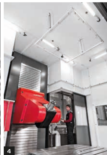
1. Thermo-symmetrical design with central head to ensure stability. 2. 4-guide column head and hydrostatic table rotation with preloaded double pinion. 3. High-precision guided LM with roller skids. 4. Integral fairing with fog extraction system. 5. Comprehensive chip and coolant collection.
